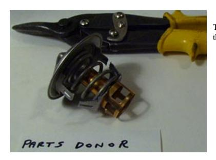
The bridge on this one does not disassemble like the Vette thermostat so the cutting began.
