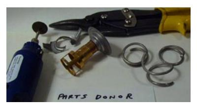
Next, the spring took two cuts so the bridge would drop down and then that got cut that too. Then two pliers were used to pull the bridge apart and remove it as shown; then the spring coils just slipped off. Care was used not to bend the diaphram or cut or damage the gold parts
