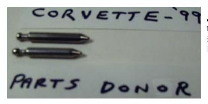
Both pins are from the top part of the thermostats. The longer one is used when re-assembling the thermostat. They are both the same diameter. When inserted, it feels like its pushing back a little from air compression. Do not worry about it, just keep going, it will settle in all the way later.
