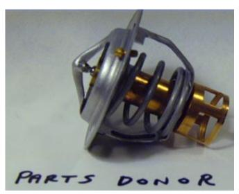
This is the parts donor. The internal gold part is what is needed and must be removed without damage. The large spring and gray housing are not needed. I have no idea what car it fits.
