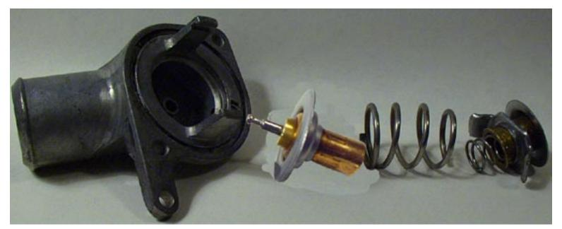
The thermostat is now ready to assemble. Notice that it looks just like the dissambled Corvette thermostat in the 2nd picture except you have removed the Corvette Diaphram (with rubber seal around the edge) and replaced it with the donor thermostat diaphram $(170^{\circ})$ .
