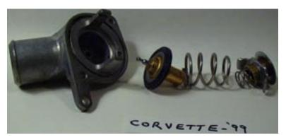
First, the Corvette thermostat was disassembled by slipping the bridge piece out from the two cast prongs. On my large spring one coil was removed (with dremel) to allow me to pry the end of the spring overtop of the bridge and rotate the spring so it would coil on top of the bridge. This relieved enough tension to enable me to push down on the bridge (with pliers and hand) and rotate it to disengage it from the prongs. This part and the reassembly were the hardest part of the mod.
